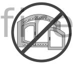
The door(s) must be closed and latched during operation. Open the door(s) only when reloading the fireplace or conducting maintenance. This prevents smoke, embers from entering the room.
