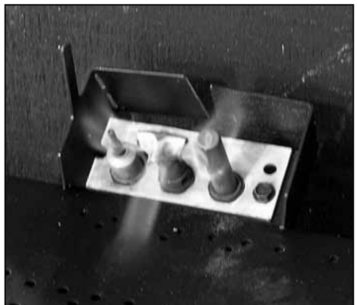
Figure 3.2 Standing Pilot Flame Patterns
