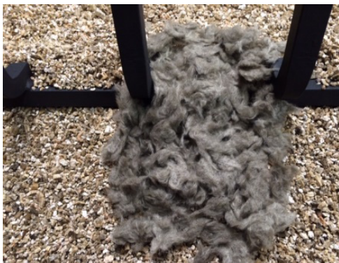
Figure 8c- Carry over tube covered by rock wool
