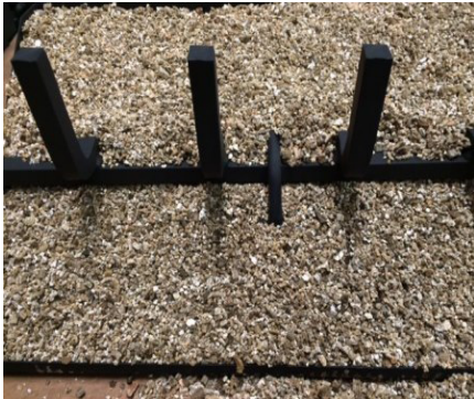
Figure 8b- Packing rock wool around the carry over tube
