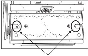
**Figure 6.1** Remove the optional brick set, if installed. Remove the two screws, one on each side of burner. Retain fasteners for reiinstallation. Lift burner up and out of the firebox.
