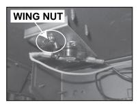
Figure 8.29 Slide temperature sensor switch/bracket assembly onto the 10-32 screw located on the left underside of the appliance. Secure the bracket assembly with the wing nut provided.
