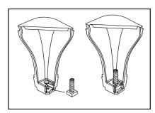
Figure 8.13 Slide assembled nuts and bolts into the slots on the legs with the nuts on the bottom.
