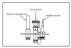
Figure 6.4 Pull off pilot hood and set aside.
