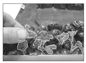
Figure 8.25 Apply dime size pieces sparingly along front edge of burner. Do not completely block ports.
