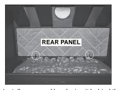
Figure 8.16 Install rear panel by placing it behind the log pins flush and centered against back of firebox.
