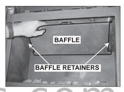
Figure 8.15 Position baffle on top of baffle retainers on left and right sides. Centering baffle on retainers, ensure that the dark painted bevelled edge and darker painted baffle bottom side faces toward the front viewing area of the firebox. Bend the center tabs up to prevent the baffle from sliding out.
