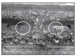
Figure 6.2 Using the #2 Phillips screwdriver remove the two (2) 1/4" x 20 screws securing the burner as indicated. Lift burner out of firebox.
