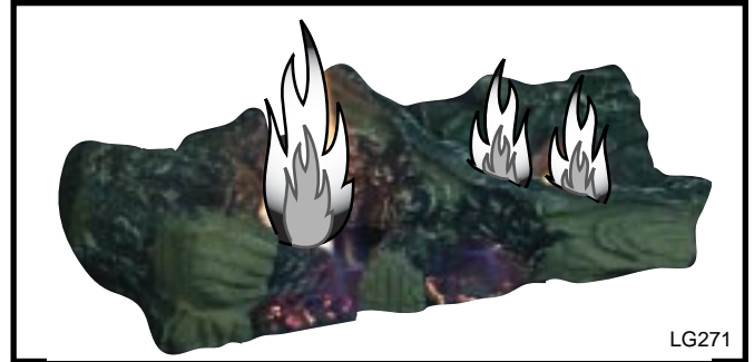
Fig. 43 Correct burner flame appearance for 33BDVT.
