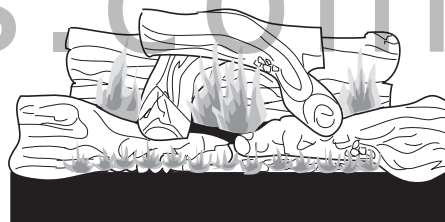
Fig. 17 Correct pilot flame pattern.
