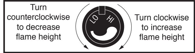
Fig. 20 Flame adjustment knob for Honeywell Valve.
