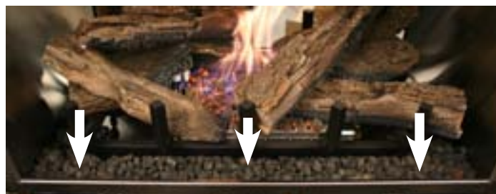
Figure 11f. Place lava rock around wrought iron grate. Place embers around burner holes. Do not cover burner holes with embers.
