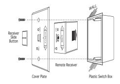
NOTE: The remote receiver will only respond to the transmitter when the 3-position slide button on the remote receiver is in the REMOTE position. If the system does not respond to the battery transmitter on initial use, see MATCHING SECURITY CODES, and recheck battery positions in the remote receiver.
