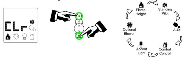
**4** With the desired mode illuminated (the illustration below shows the AUX mode illuminated), press the "up" or "down" button to activate or clear the mode being addressed. Make sure to keep the on/off button depressed during this process.
