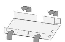
Attach the two pieces of double-sided tape to the bracket. Place the receiver as shown on top of the tape.
