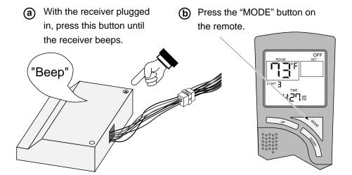
The remote will beep five times to indicate the receiver is calibrated.
