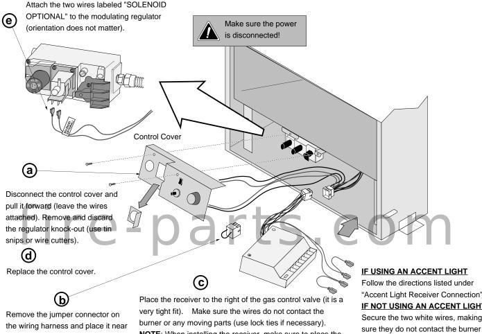
the gas control valve (it is required if you wish to remove the remote). Attach the molex connector from the receiver to the molex connector on the appliance.
