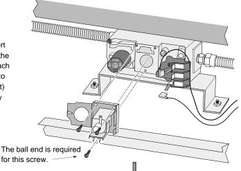
Attach the two remote on/off wires (red and brown) from the wiring harness to the top and bottom terminals on the gas control valve (orientation does not matter).
